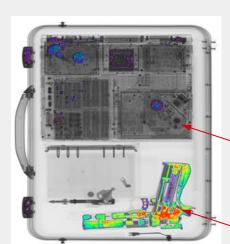
The camera can detect different metal materials within bags and it allows even more accurate identification during baggage/luggage inspection.
